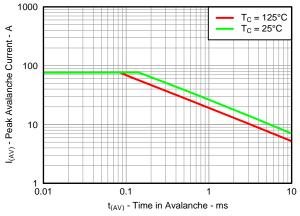
Figure 11. Single Pulse Unclamped Inductive Switching
