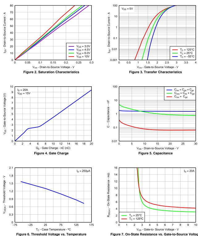
Figure 7. On-State Resistance vs. Gate-to-Source Voltage
