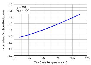
Figure 8. Normalized On-State Resistance vs. Temperature
