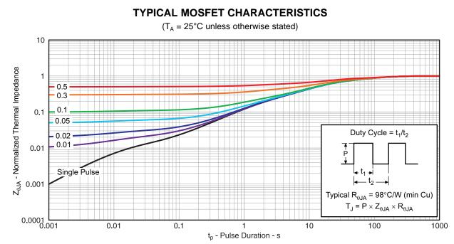
Figure 1. Transient Thermal Impedance
