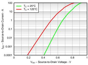
Figure 9. Typical Diode Forward Voltage
