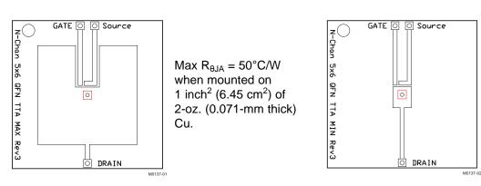
Max  $R_{\theta,JA} = 120^{\circ}C/W$ when mounted on a minimum pad area of 2-oz. (0.071-mm thick) Cu.
