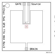
Max  $R_{\theta JA} = 50^{\circ}\text{C/W}$  when mounted on 1 inch² (6.45 cm²) of 2-oz. (0.071-mm thick) Cu.
