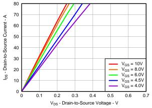
Figure 2. Saturation Characteristics
