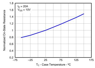
Figure 8. Normalized On-State Resistance vs. Temperature
