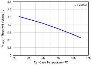
Figure 6. Threshold Voltage vs. Temperature
