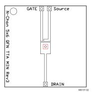
Max  $R_{\theta JA} = 120^{\circ} C/W$  when mounted on a minimum pad area of 2-oz. (0.071-mm thick) Cu.
