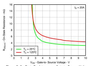
Figure 7. On-State Resistance vs. Gate-to-Source Voltage
