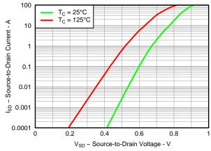
Figure 9. Typical Diode Forward Voltage
