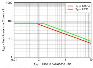
Figure 11. Single Pulse Unclamped Inductive Switching
