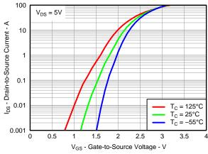
Figure 3. Transfer Characteristics
