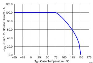
Figure 12. Maximum Drain Current vs. Temperature
