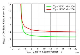
Figure 7. On-State Resistance vs. Gate-to-Source Voltage
