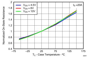
Figure 8. Normalized On-State Resistance vs. Temperature
