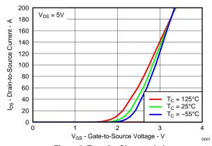
Figure 3. Transfer Characteristics
