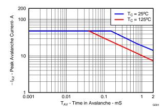
Figure 11. Single Pulse Unclamped Inductive Switching
