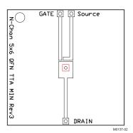
Max  $R_{\theta JA} = 122.4^{\circ} C/W$  when mounted on a minimum pad area of 2-oz. (0.071-mm thick) Cu.
