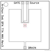
Max  $R_{\theta JA} = 50.6^{\circ}\text{C/W}$  when mounted on 1 inch² (6.45-cm²) of 2-oz. (0.071-mm thick) Cu.
