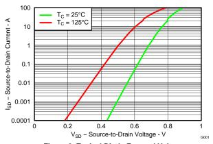
Figure 9. Typical Diode Forward Voltage
