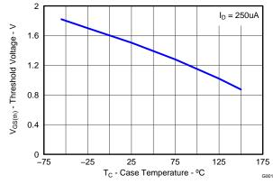
Figure 6. Threshold Voltage vs. Temperature
