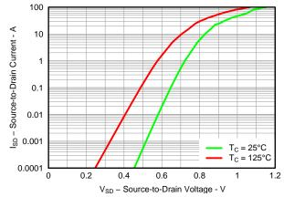
Figure 24. Control MOSFET Body Diode
