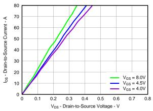
Figure 11. Sync MOSFET Saturation
