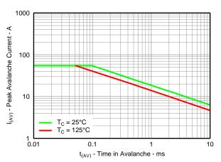
Figure 27. Sync MOSFET Unclamped Inductive Switching
