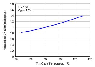
Figure 22. Control MOSFET Normalized R<sub>DS(on)</sub>
