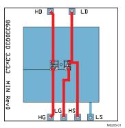
Max  $R_{\theta JA} = 73^{\circ} C/W$  when mounted on 1 inch² (6.45 cm²) of 2-oz. (0.071-mm thick) Cu.
