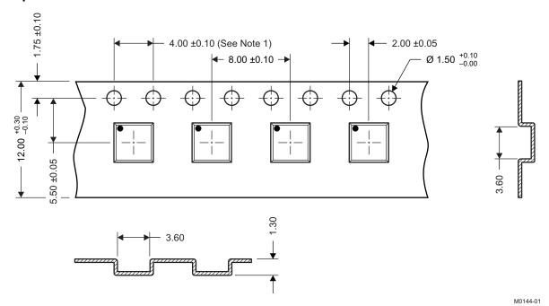
NOTES: 1. 10-sprocket hole-pitch cumulative tolerance ±0.2
