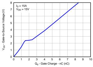
Figure 14. Control MOSFET Gate Charge
