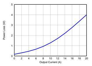
Figure 1. Power Loss vs Output Current
