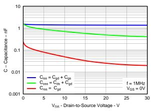
Figure 17. Sync MOSFET Capacitance
