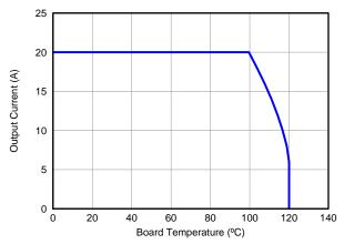
Figure 5. Typical Safe Operating Area<sup>(1)</sup>
