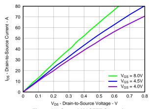
Figure 10. Control MOSFET Saturation
