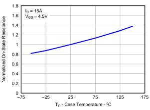
Figure 23. Sync MOSFET Normalized R<sub>DS(on)</sub>
