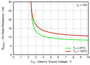
Figure 20. Control MOSFET R<sub>DS(on)</sub> vs V<sub>GS</sub>
