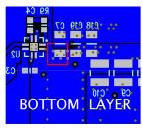
Figure 34. Recommended PCB Layout (Top Down)
