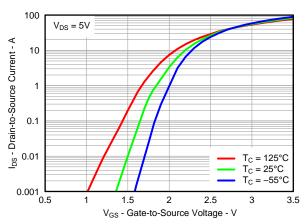
Figure 12. Control MOSFET Transfer
