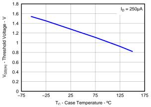
Figure 18. Control MOSFET V<sub>GS(th)</sub>
