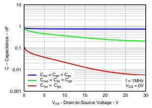
Figure 16. Control MOSFET Capacitance
