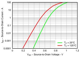
Figure 25. Sync MOSFET Body Diode
