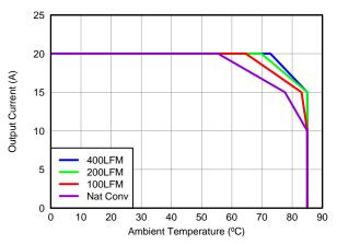
Figure 4. Safe Operating Area – PCB Horizontal Mount<sup>(1)</sup>
