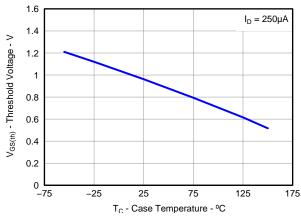
Figure 19. Sync MOSFET V<sub>GS(th)</sub>
