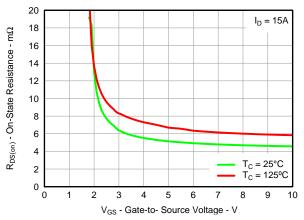
Figure 21. Sync MOSFET R<sub>DS(on)</sub> vs V<sub>GS</sub>
