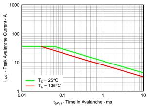
Figure 26. Control MOSFET Unclamped Inductive Switching
