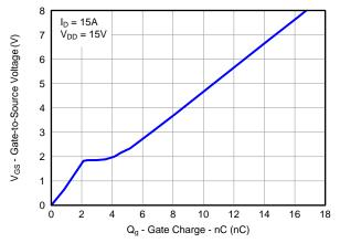
Figure 15. Sync MOSFET Gate Charge
