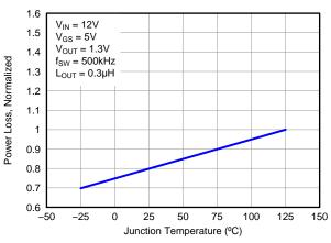
Figure 2. Normalized Power Loss vs Temperature
