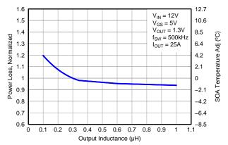
Figure 9. Normalized Power Loss vs. Output Inductance
