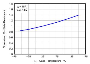
Figure 22. Control MOSFET Normalized R<sub>DS(on)</sub>
