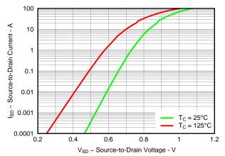
Figure 24. Control MOSFET Body Diode
