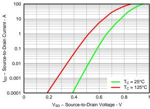
Figure 25. Sync MOSFET Body Diode
