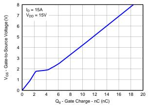
Figure 15. Sync MOSFET Gate Charge
