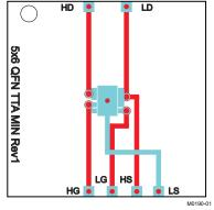
Max  $R_{\theta JA} = 150$  °C/W when mounted on minimum pad area of 2-oz. (0.071-mm thick) Cu.
