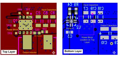
Figure 34. Recommended PCB Layout (Top Down View)
