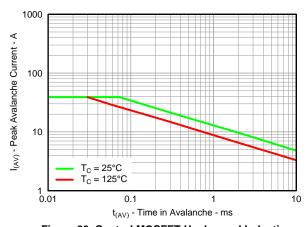
Figure 26. Control MOSFET Unclamped Inductive Switching
