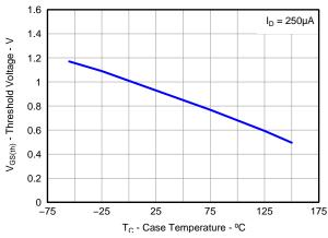
Figure 19. Sync MOSFET V<sub>GS(th)</sub>
