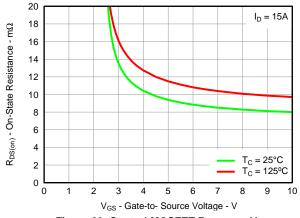
Figure 20. Control MOSFET R<sub>DS(on)</sub> vs V<sub>GS</sub>
