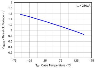
Figure 18. Control MOSFET V<sub>GS(th)</sub>
