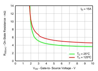
Figure 21. Sync MOSFET R<sub>DS(on)</sub> vs V<sub>GS</sub>
