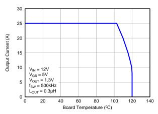
Figure 5. Typical Safe Operating Area<sup>(1)</sup>
