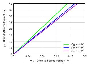
Figure 11. Sync MOSFET Saturation
