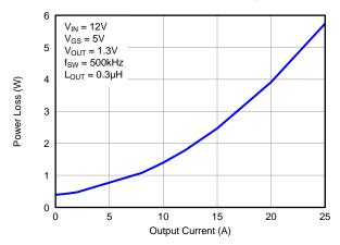
Figure 1. Power Loss vs Output Current
