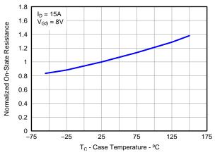
Figure 23. Sync MOSFET Normalized R<sub>DS(on)</sub>
