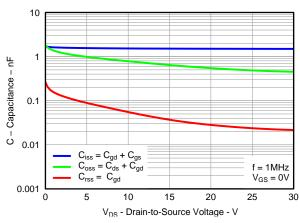
Figure 17. Sync MOSFET Capacitance
