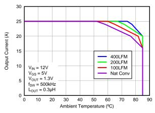
Figure 3. Safe Operating Area – PCB Vertical Mount<sup>(1)</sup>
