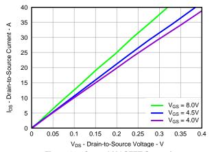
Figure 10. Control MOSFET Saturation
