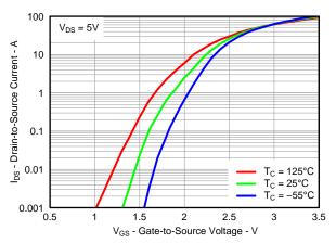
Figure 12. Control MOSFET Transfer
