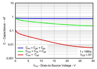
Figure 16. Control MOSFET Capacitance
