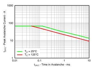
Figure 27. Sync MOSFET Unclamped Inductive Switching
