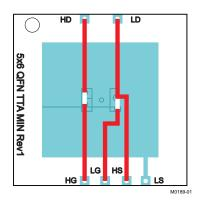
Max  $R_{\theta JA} = 82^{\circ}\text{C/W}$  when mounted on 1 inch<sup>2</sup> (6.45 cm<sup>2</sup>) of 2-oz. (0.071-mm thick) Cu.
