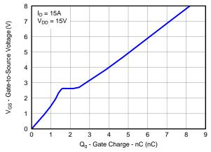
Figure 14. Control MOSFET Gate Charge
