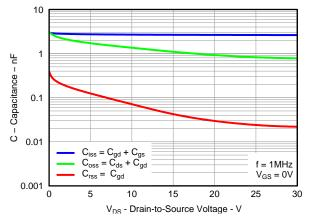
Figure 16. Control MOSFET Capacitance
