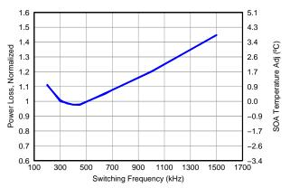
Figure 6. Normalized Power Loss vs Switching Frequency
