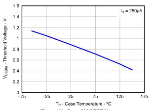
Figure 19. Sync MOSFET V<sub>GS(th)</sub>
