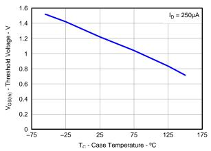
Figure 18. Control MOSFET V<sub>GS(th)</sub>
