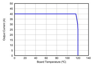
Figure 5. Typical Safe Operating Area<sup>(1)</sup>
