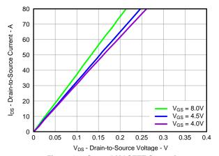
Figure 10. Control MOSFET Saturation
