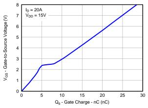
Figure 14. Control MOSFET Gate Charge
