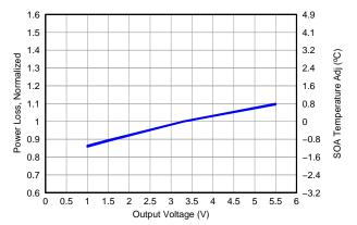
Figure 8. Normalized Power Loss vs. Output Voltage
