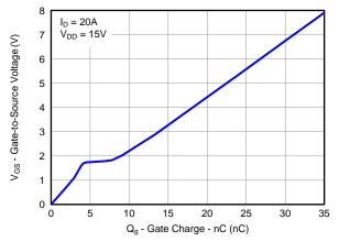
Figure 15. Sync MOSFET Gate Charge
