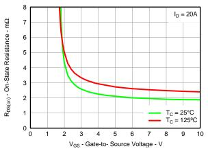
Figure 21. Sync MOSFET R<sub>DS(on)</sub> vs V<sub>GS</sub>
