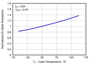
Figure 23. Sync MOSFET Normalized R<sub>DS(on)</sub>
