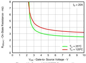
Figure 20. Control MOSFET R<sub>DS(on)</sub> vs V<sub>GS</sub>
