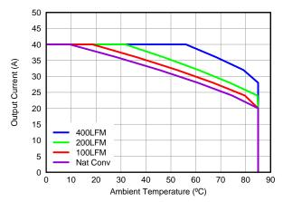
Figure 3. Safe Operating Area – PCB Vertical Mount<sup>(1)</sup>
