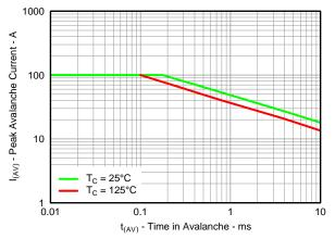
Figure 27. Sync MOSFET Unclamped Inductive Switching
