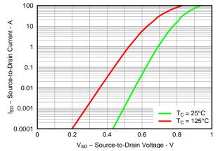
Figure 24. Control MOSFET Body Diode
