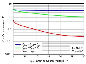
Figure 17. Sync MOSFET Capacitance
