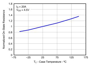
Figure 22. Control MOSFET Normalized R<sub>DS(on)</sub>
