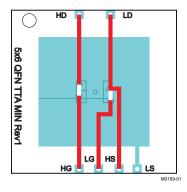
Max  $R_{\theta JA} = 50^{\circ} C/W$  when mounted on 1 inch<sup>2</sup> (6.45 cm<sup>2</sup>) of 2-oz. (0.071-mm thick) Cu.
