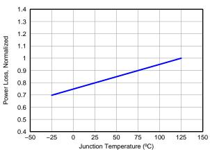
Figure 2. Normalized Power Loss vs Temperature
