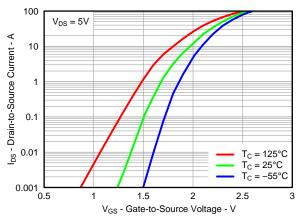
Figure 12. Control MOSFET Transfer
