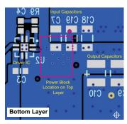
Figure 34. Recommended PCB Layout (Top Down View)
