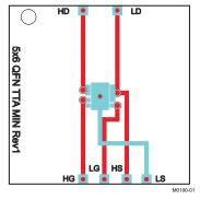
Max  $R_{\theta JA} = 102^{\circ} C/W$  when mounted on minimum pad area of 2-oz. (0.071-mm thick) Cu.
