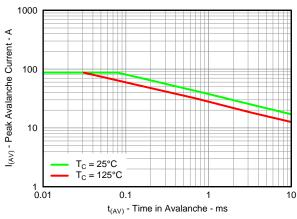
Figure 26. Control MOSFET Unclamped Inductive Switching
