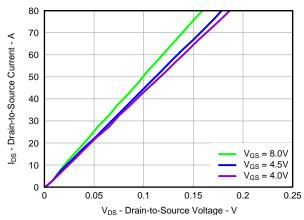
Figure 11. Sync MOSFET Saturation
