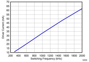
Figure 16. Driver Current vs Frequency
