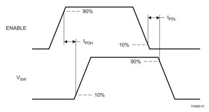
Figure 5. CSD97370Q5M ENABLE Timing Diagram ( $V_{DD} = PWM = 5V$ )
