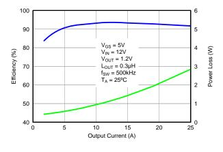
Figure 2. Efficiency and Power Loss
