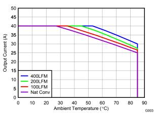
Figure 9. Safe Operating Area – PCB Vertical Mount (1)
