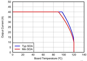
Figure 11. Typical and Min Safe Operating Area (1)
