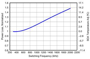
Figure 12. Normalized Power Loss vs Frequency
