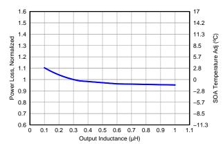
Figure 15. Normalized Power Loss vs Output Inductance
