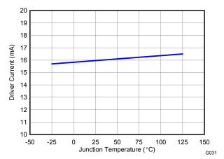
Figure 17. Driver Current vs Temperature
