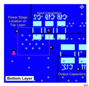
Figure 20. Recommended PCB Layout (Top Down View)
