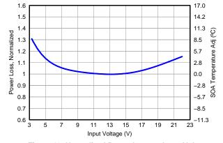
Figure 13. Normalized Power Loss vs Input Voltage
