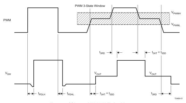
Figure 6. CSD97370Q5M PWM Timing Diagram
