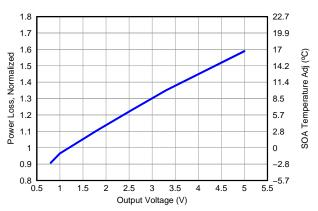
Figure 14. Normalized Power Loss vs Output Voltage
