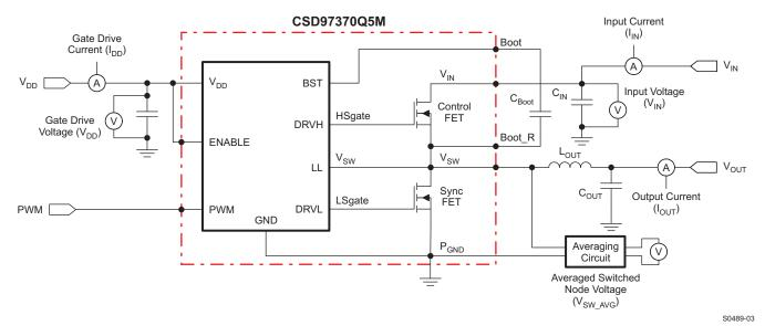
Figure 18. Power Loss Test Circuit
