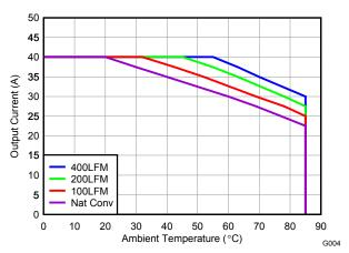
Figure 10. Safe Operating Area – PCB Horizontal Mount (1)
