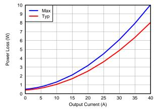
Figure 7. Power Loss vs Output Current
