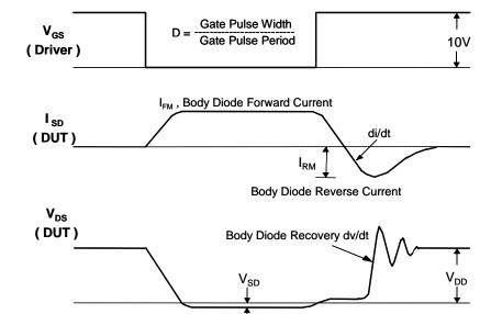
Body Diode Forward Voltage Drop
