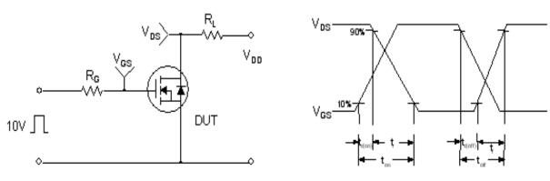
**Unclamped Inductive Switching Test Circuit & Waveforms**
