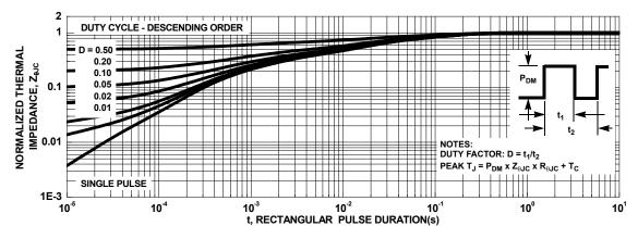
Figure 3. Normalized Maximum Transient Thermal Impedance
