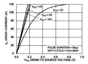
Figure 7. Transfer Characteristics
