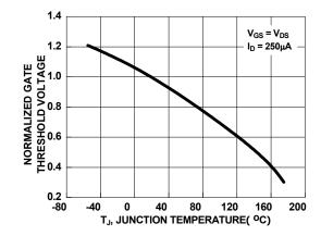
Figure 11. Normalized Gate Threshold Voltage vs
