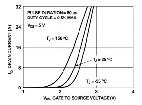
Figure 5. Transfer Characteristics
