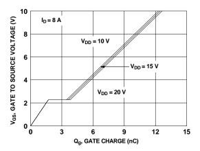
Figure 7. Gate Charge Characteristics
