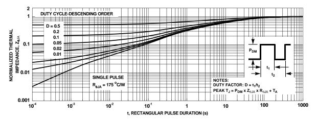
Figure 13. Junction-to-Ambient Transient Thermal Response Curve
