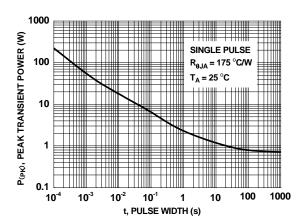
Figure 12. Single Pulse Maximum Power Dissipation
