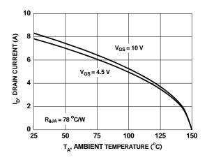
Figure 10. Maximum Continous Drain Current vs. Ambient Temperature
