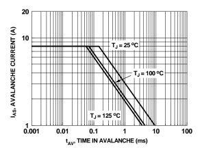
Figure 9. Unclamped Inductive Switching Capability
