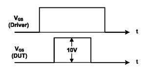
$$Qsync = \frac{1}{R_G} \cdot \int V_{R_G}(t) dt$$
