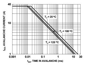
Figure 9. Unclamped Inductive Switching Capability
