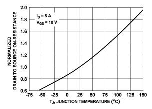
Figure 3. Normalized On-Resistance vs Junction Temperature
