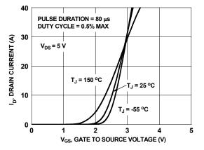
Figure 5. Transfer Characteristics
