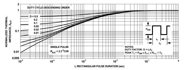
Figure 14. Junction-to-Case Transient Thermal Response Curve
