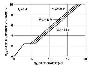
Figure 7. Gate Charge Characteristics
