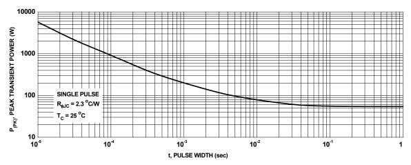
Figure 13. Single Pulse Maximum Power Dissipation
