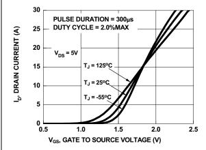
Figure 5. Transfer Characteristics
