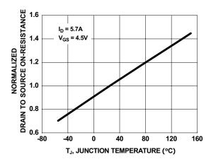
Figure 3. Normalized On Resistance vs Junction Temperature
