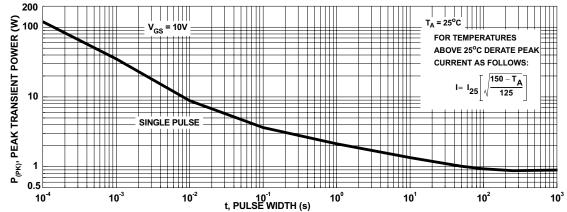
Figure 11. Single Pulse Maximum Power Dissipation
