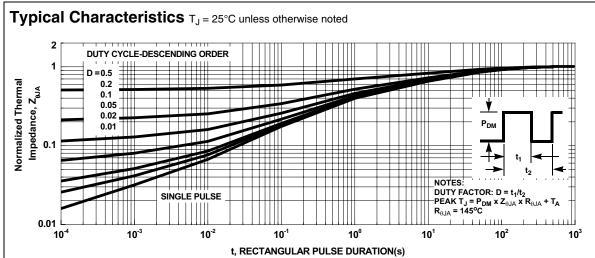
Figure 12. Transient Thermal Response Curve
