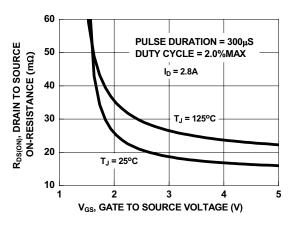
Figure 4. On-Resistance vs Gate to Source Votlage
