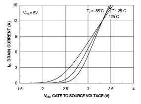
Figure 5. Transfer Characteristics
