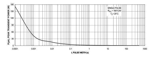
Figure 11. Single Pulse Maximum Power Dissipation
