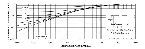
Figure 12. Transient Thermal Response Curve
