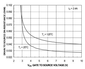
Figure 4. On-Resistance vs Gate to Source Voltage
