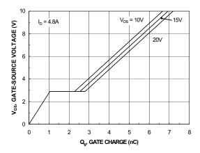
Figure 7. Gate Charge Characteristics
