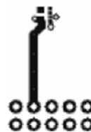
b. 165\text{ }^\circ\text{C/W} when mounted on a minimum pad of 2 oz copper
