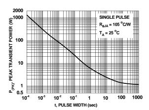
Figure 12. Single Pulse Maximum Power Dissipation
