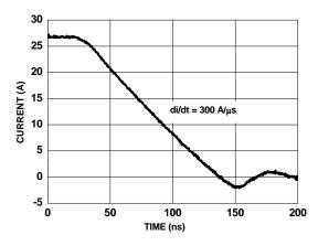
Figure 14. FDMC2512SDC SyncFET body diode reverse recovery characteristic
