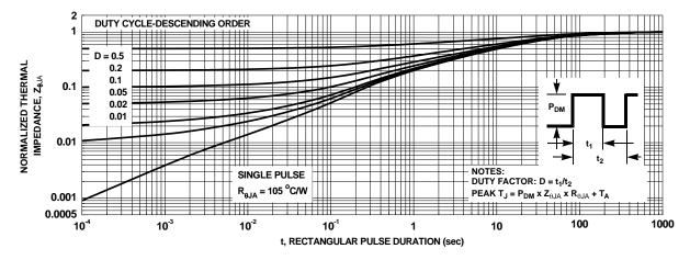
Figure 13. Junction-to-Ambient Transient Thermal Response Curve
