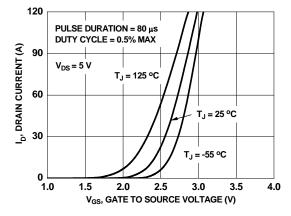
Figure 5. Transfer Characteristics
