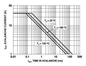
Figure 9. Unclamped Inductive Switching Capability
