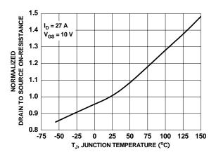
Figure 3. Normalized On-Resistance vs Junction Temperature
