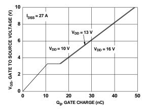
Figure 7. Gate Charge Characteristics
