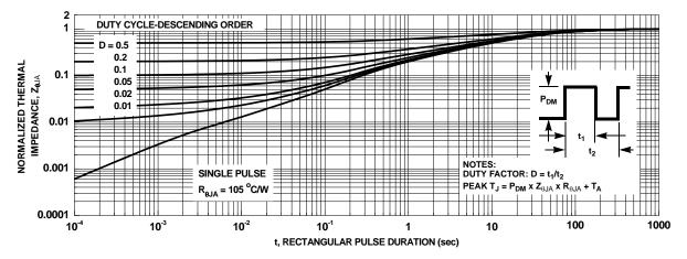
Figure 13. Junction-to-Ambient Transient Thermal Response Curve
