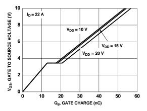
Figure 7. Gate Charge Characteristics
