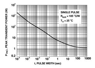
Figure 12. Single Pulse Maximum Power Dissipation
