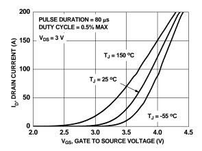
Figure 5. Transfer Characteristics
