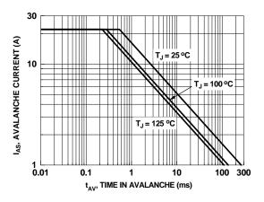
Figure 9. Unclamped Inductive Switching Capability
