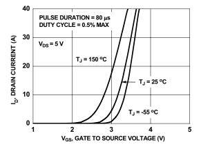
Figure 5. Transfer Characteristics
