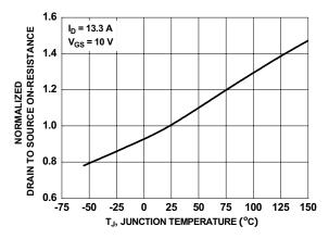
Figure 3. Normalized On-Resistance vs Junction Temperature
