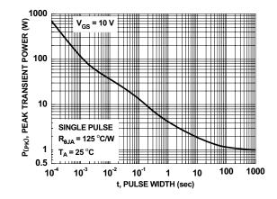
Figure 12. Single Pulse Maximum Power Dissipation
