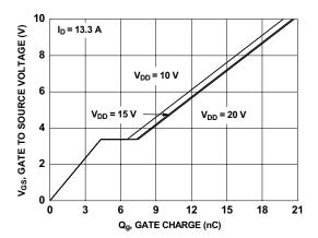
Figure 7. Gate Charge Characteristics
