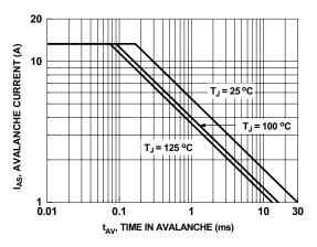
Figure 9. Unclamped Inductive Switching Capability
