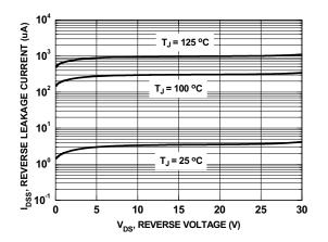
Figure 14. SyncFET body diode reverses leakage versus drain-source voltage
