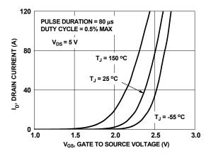
Figure 5. Transfer Characteristics
