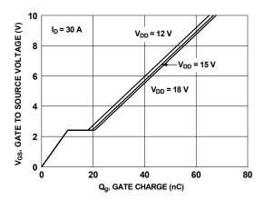
Figure 7. Gate Charge Characteristics
