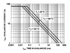
Figure 9. Unclamped Inductive Switching Capability
