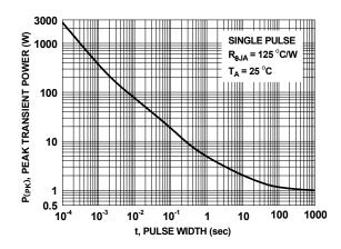
Figure 12. Single Pulse Maximum Power Dissipation
