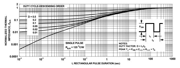
Figure 13. Junction-to-Ambient Transient Thermal Response Curve
