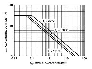
Figure 9. Unclamped Inductive Switching Capability
