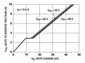
Figure 7. Gate Charge Characteristics
