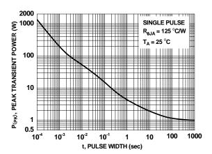
Figure 12. Single Pulse Maximum Power Dissipation
