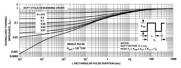
Figure 13. Junction-to-Ambient Transient Thermal Response Curve
