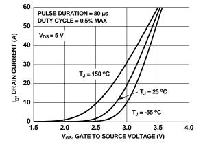
Figure 5. Transfer Characteristics
