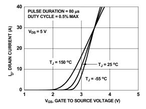
Figure 5. Transfer Characteristics
