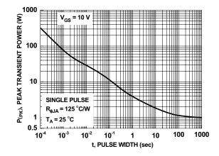
Figure 12. Single Pulse Maximum Power Dissipation
