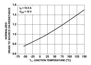
Figure 3. Normalized On-Resistance vs Junction Temperature
