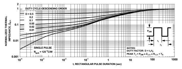
Figure 13. Transient Thermal Response Curve
