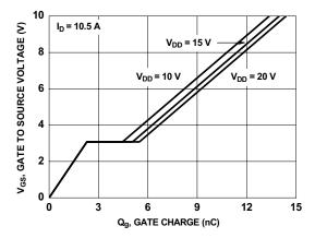
Figure 7. Gate Charge Characteristics
