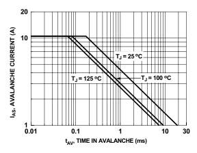
Figure 9. Unclamped Inductive Switching Capability
