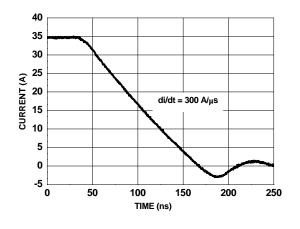
Figure 14. FDMS2502SDC SyncFET body diode reverse recovery characteristic
