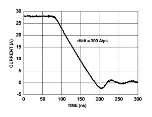
Figure 14. FDMS3008SDC SyncFET body diode reverse recovery characteristic
