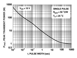
Figure 12. Single Pulse Maximum Power Dissipation
