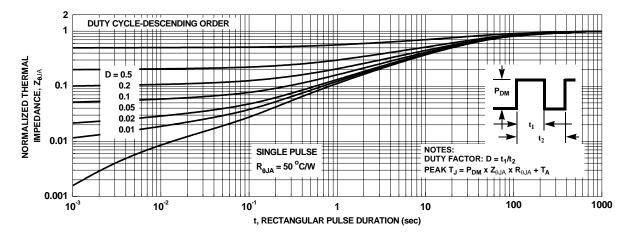
Figure 13. Junction-to-Ambient Transient Thermal Response Curve
