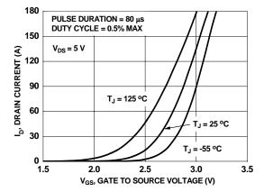
Figure 5. Transfer Characteristics
