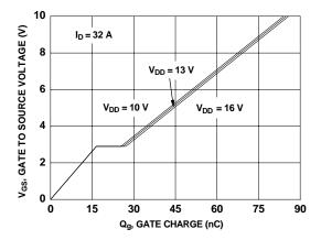
Figure 7. Gate Charge Characteristics
