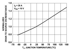
Figure 3. Normalized On-Resistance vs Junction Temperature
