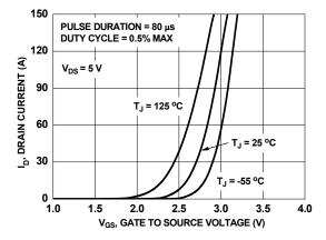
Figure 5. Transfer Characteristics
