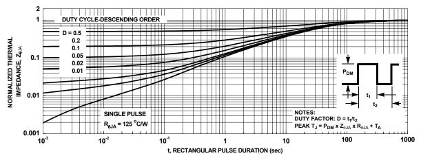
Figure 13. Junction-to-Ambient Transient Thermal Response Curve
