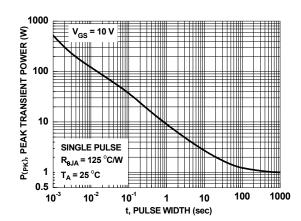
Figure 12. Single Pulse Maximum Power Dissipation
