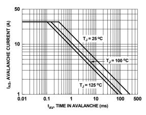
Figure 9. Unclamped Inductive Switching Capability
