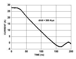
Figure 14. FDMS7658AS SyncFET body diode reverse recovery characteristic
