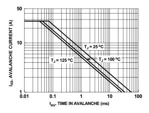
Figure 9. Unclamped Inductive Switching Capability
