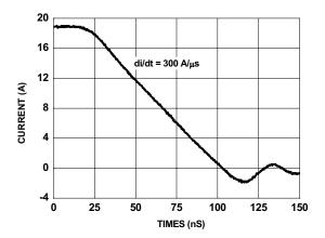
Figure 14. Body Diode Reverse Recovery Characteristics
