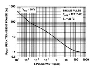
Figure 12. Single Pulse Maximum Power Dissipation
