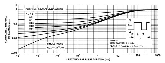
Figure 13. Junction-to-Ambient Transient Thermal Response Curve
