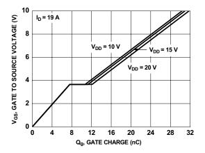
Figure 7. Gate Charge Characteristics
