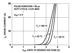
Figure 5. Transfer Characteristics
