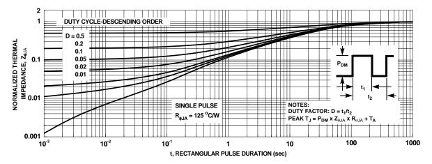
Figure 13. Junction-to-Ambient Transient Thermal Response Curve
