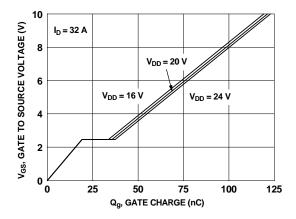
Figure 7. Gate Charge Characteristics
