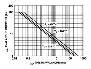
Figure 9. Unclamped Inductive Switching Capability
