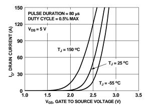
Figure 5. Transfer Characteristics
