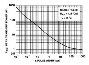
Figure 12. Single Pulse Maximum Power Dissipation
