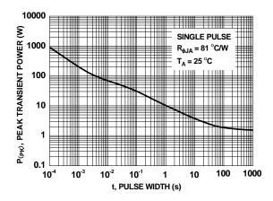
Figure 12. Single Pulse Maximum Power Dissipation
