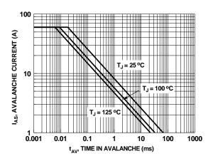
Figure 9. Unclamped Inductive Switching Capability
