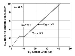
Figure 7. Gate Charge Characteristics
