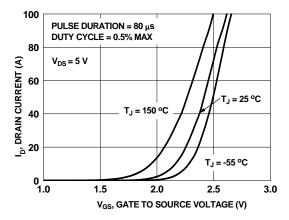
Figure 5. Transfer Characteristics
