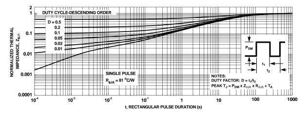
Figure 13. Junction-to-Ambient Transient Thermal Response Curve
