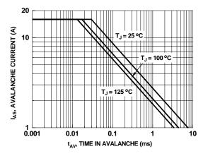
Figure 9. Unclamped Inductive Switching Capability
