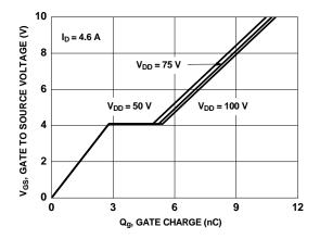
Figure 7. Gate Charge Characteristics
