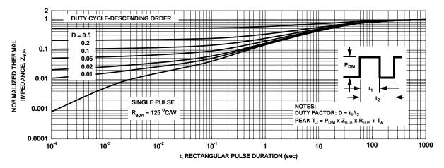
Figure 13. Junction-to-Ambient Transient Thermal Response Curve
