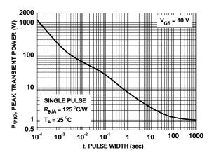
Figure 12. Single Pulse Maximum Power Dissipation
