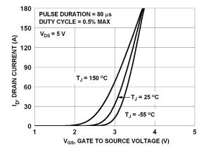
Figure 5. Transfer Characteristics
