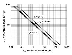
Figure 9. Unclamped Inductive Switching Capability
