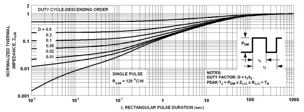
Figure 13. Junction-to-Ambient Transient Thermal Response Curve
