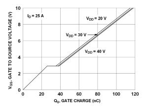
Figure 7. Gate Charge Characteristics
