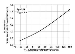
Figure 3. Normalized On-Resistance vs Junction Temperature
