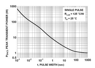
Figure 12. Single Pulse Maximum Power Dissipation
