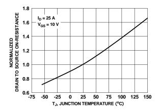
Figure 3. Normalized On-Resistance vs Junction Temperature
