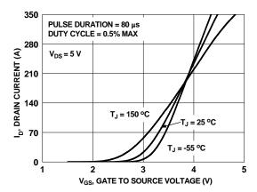
Figure 5. Transfer Characteristics
