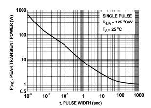
Figure 12. Single Pulse Maximum Power Dissipation
