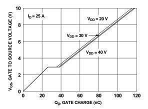
Figure 7. Gate Charge Characteristics
