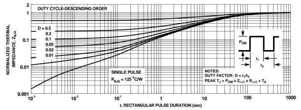
Figure 13. Junction-to-Ambient Transient Thermal Response Curve
