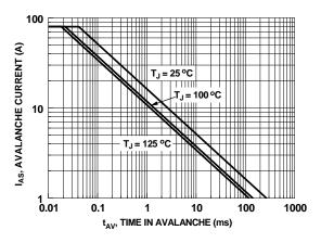
Figure 9. Unclamped Inductive Switching Capability
