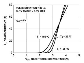
Figure 5. Transfer Characteristics
