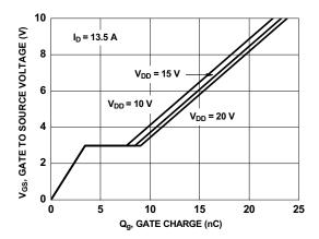
Figure 7. Gate Charge Characteristics
