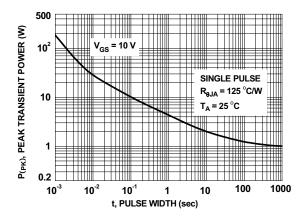
Figure 12. Single Pulse Maximum Power Dissipation
