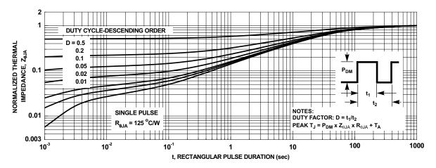
Figure 13. Junction-to-Ambient Transient Thermal Response Curve
