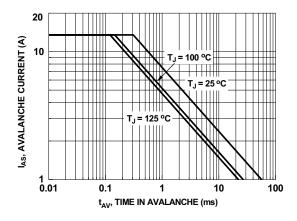
Figure 9. Unclamped Inductive Switching Capability
