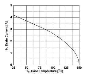
Figure 8. Maximum Safe Operating Area vs. Case Temperature-FDPF5N50NZF
