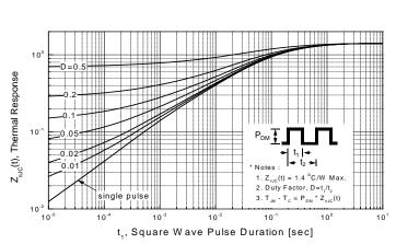
Figure 10-1. Transient Thermal Response Curve - FDP7N50U
