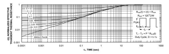
Figure 11. Transient Thermal Response Curve.
