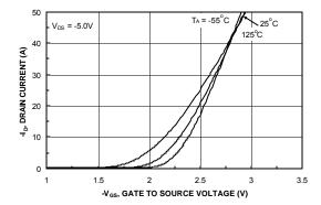
Figure 5. Transfer Characteristics.
