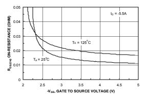
Figure 4. On-Resistance Variation with Gate-to-Source Voltage.
