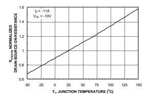
Figure 3. On-Resistance Variation with Temperature.
