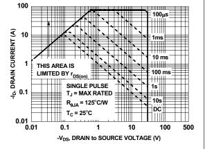
Figure 11. Maximum Continuous Drain Current vs
