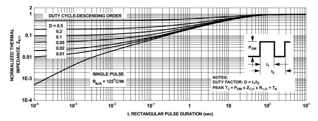
Figure 14. Junction-to-Ambient Transient Thermal Response Curve
