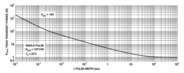
Figure 13. Single Pulse Maximum Power Dissipation
