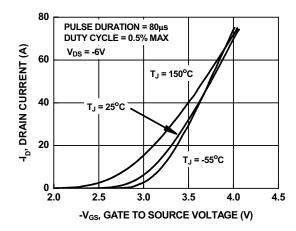
Figure 5. Transfer Characteristics
