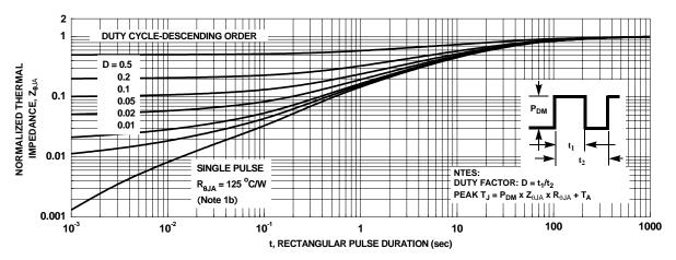
Figure 13. Junction-to-Ambient Transient Thermal Response Curve
