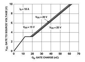
Figure 7. Gate Charge Characteristics
