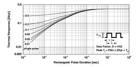
Figure 22. Transient Thermal Impedance of Diode
