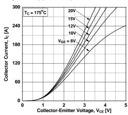
Figure 4. Saturation Voltage vs. Case
