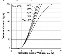
Figure 3. Typical Saturation Voltage Characteristics
