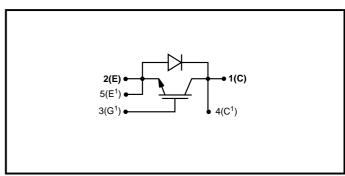
Fig. 1 Single switch circuit diagram
