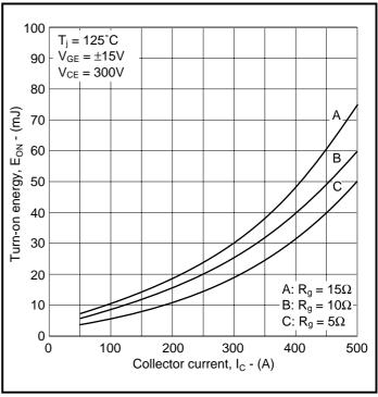
Fig.6 Typical turn-on energy vs collector current
