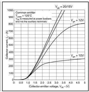
Fig.3 Typical output characteristics
