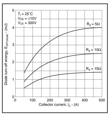
Fig.9 Typical diode turn-off energy vs collector current
