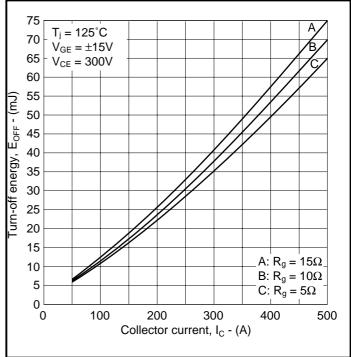
Fig.7 Typical turn-off energy vs collector current
