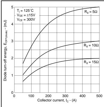
Fig.10 Typical diode turn-off energy vs collector current
