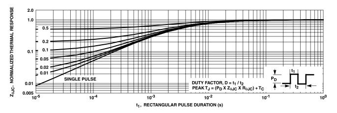
FIGURE 17. NORMALIZED TRANSIENT THERMAL RESPONSE, JUNCTION TO CASE
