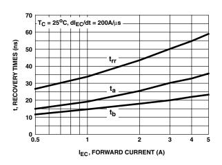
FIGURE 19. RECOVERY TIMES vs FORWARD CURRENT
