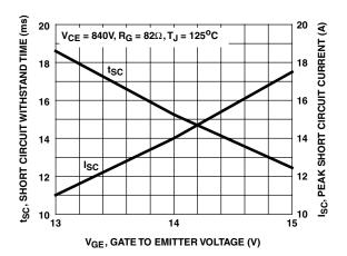
FIGURE 4. SHORT CIRCUIT WITHSTAND TIME
