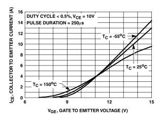
FIGURE 13. TRANSFER CHARACTERISTIC
