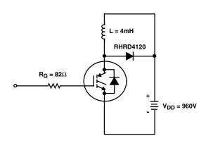
FIGURE 20. INDUCTIVE SWITCHING TEST CIRCUIT
