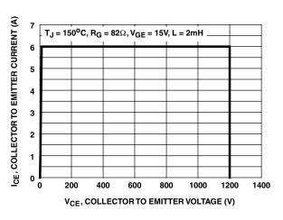
FIGURE 2. MINIMUM SWITCHING SAFE OPERATING AREA
