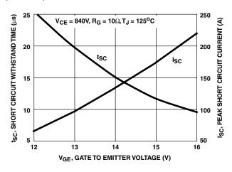
FIGURE 4. SHORT CIRCUIT WITHSTAND TIME
