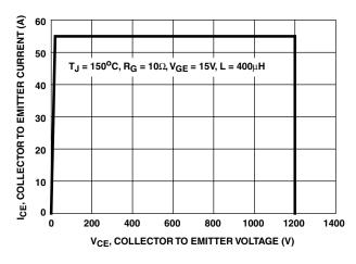
FIGURE 2. MINIMUM SWITCHING SAFE OPERATING AREA
