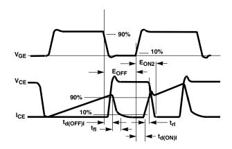
FIGURE 19. SWITCHING TEST WAVEFORMS
