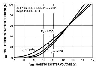
FIGURE 13. TRANSFER CHARACTERISTIC
