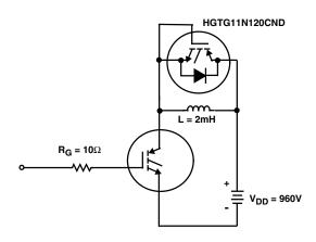
FIGURE 18. INDUCTIVE SWITCHING TEST CIRCUIT
