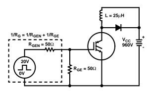
FIGURE 12. INDUCTIVE SWITCHING TEST CIRCUIT
