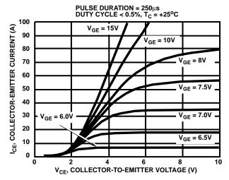
FIGURE 2. SATURATION CHARACTERISTICS (TYPICAL)
