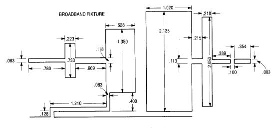
Figure 1. Test Circuit
