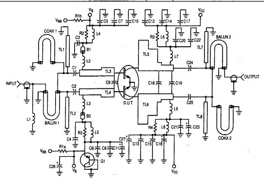
B1, B2 - Ferrite Bead, Ferroxcube #56--590-65-3B C1, C2, C24, C25 - 43 pF, B Case, ATC Chip Capacitor C3, C4, C20, C21 — 100 pF, B Case, ATC Chip Capacitor C5, C6, C12, C13 — 1000 pF, B Case, ATC Chip Capacitor C7, C8, C14, C15 — 1800 pF, AVX Chip Capacitor C9 - 9.1 pF, A Case, ATC Chip Capacitor C10, C11, C17, C18, C22, C23 - 10 µF, Electrolytic Capacitor Panasonic C16 — 3.9 pF, B Case, ATC Chip Capacitor C19 — 0.8 pF, B Case, ATC Chip Capacitor
