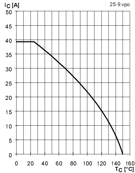
Fig. 8 Rated current vs. temperature I_C = f(T_C)
