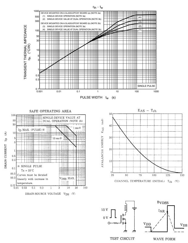
$T_{ch}=25^{\circ}C$  (Initial)  $\begin{array}{l} T_{ch} = 25^{\circ}C \ (Initial) \\ Peak \ IAR = 4.5 \ A, \ R_G = 25 \ \Omega \quad EAS = \frac{1}{2} \cdot L \cdot I^2 \cdot \ (\frac{BVDSS}{BVDSS - V_{DD}}) \end{array}$
