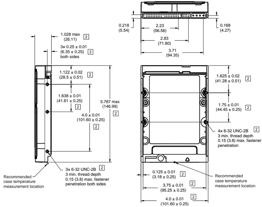
**Figure 4. Mounting dimensions—top, side and end view**
